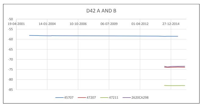
Figure 4.67 Water levels in D42A and D42B in mbgl
