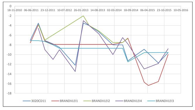
Figure 4.17 Groundwater levels in D57A (3020CD11) and D57B (Brandvlei) in mbgl
